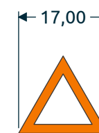
DETAIL C | TACTILE WARNING SCALE 1 : 1
