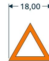
DETAIL C | TACTILE WARNING SCALE 1 : 1
