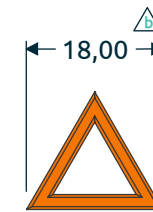
DETAIL C | TACTILE WARNING SCALE 1:1
